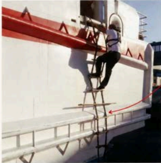
Example: Inadequately rigged pilot ladder on a ferry. This arrangement is unsafe and non-compliant.
