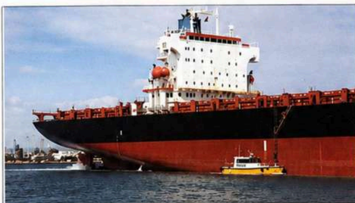
Combination ladder arrangement on a vessel with freeboard > 9 m
