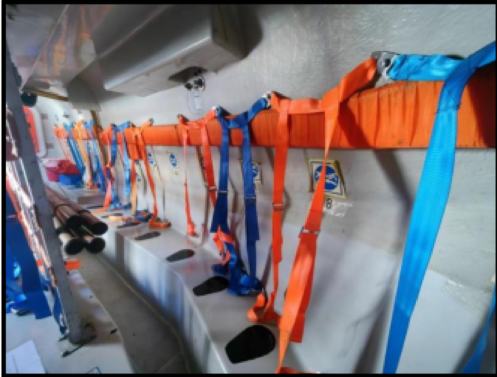
Lifeboat safety belt partly missing
