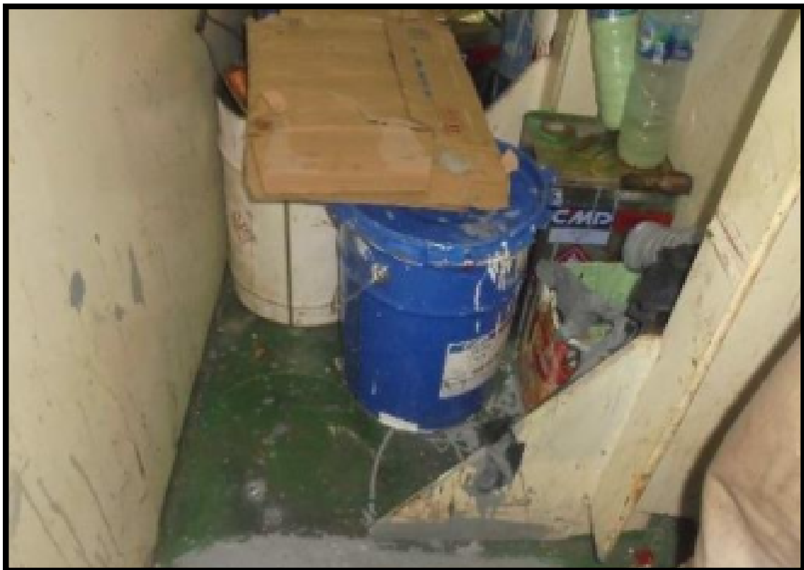
Improper stowage of flammable material in accommodation
