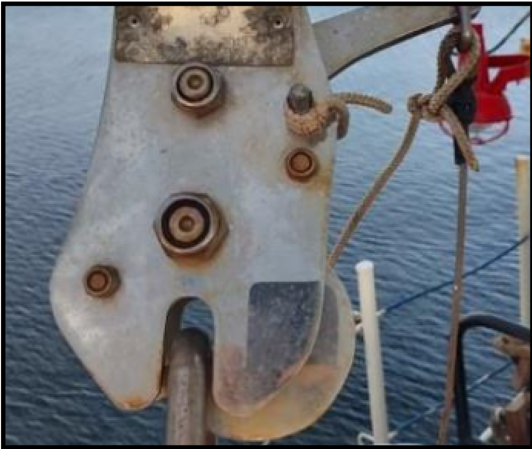
Usage of unapproved life raft hook
