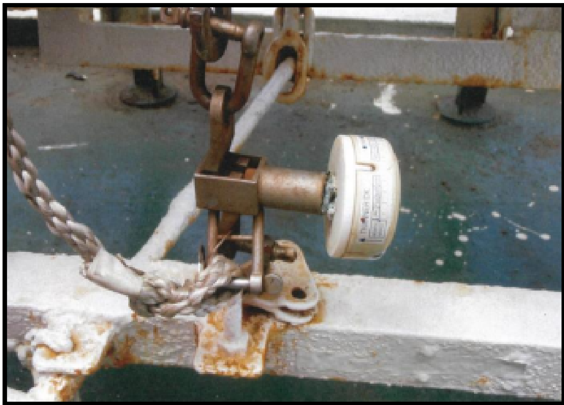
Damaged hydrostatic release unit
