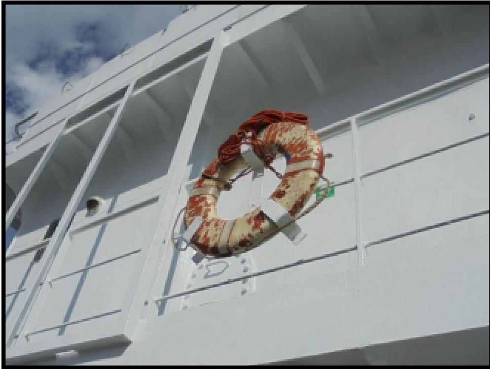
Peeling paint on lifebuoy
