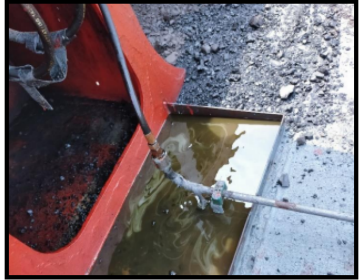
Leakage from the on board hydraulic system
