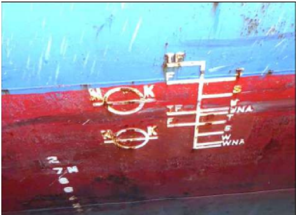
Improper freeboard marks
