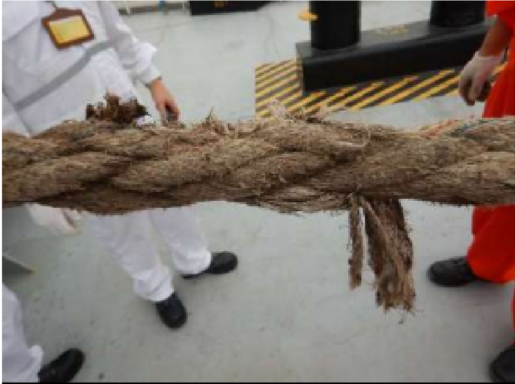
Partly broken mooring rope
