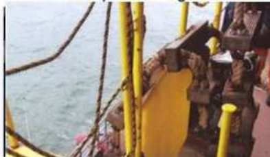
Seizing with strong twine above and below the step.
