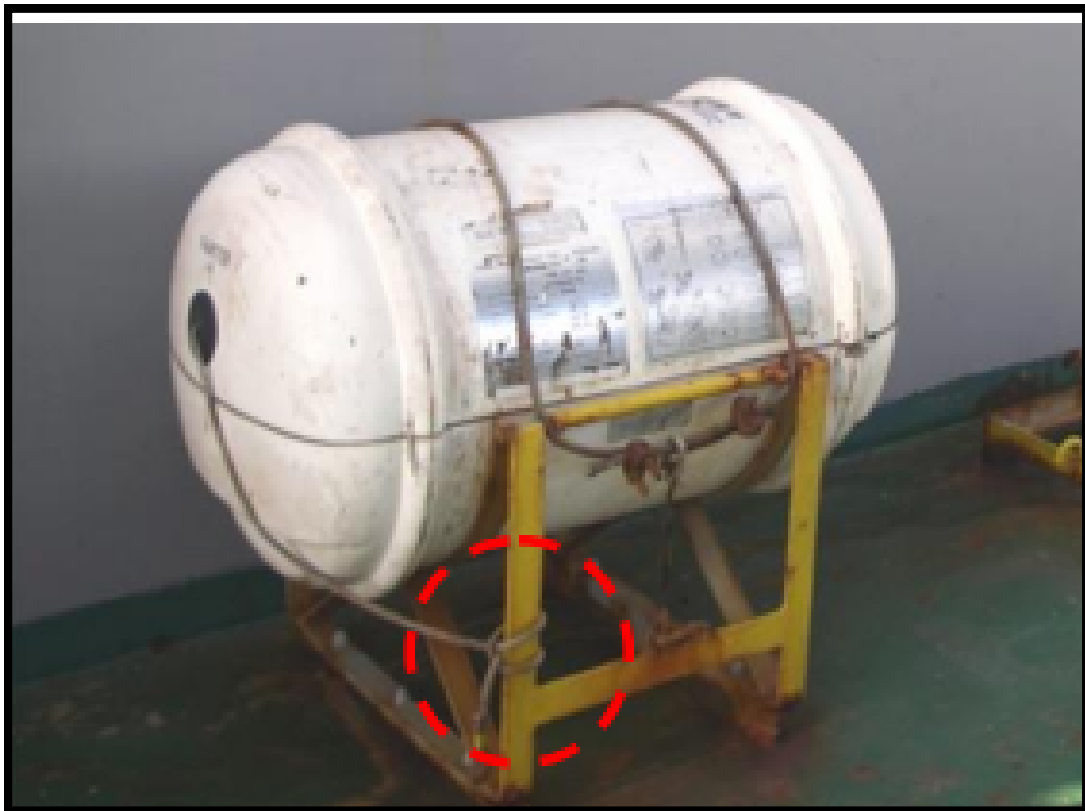
Inappropriate painter securing
