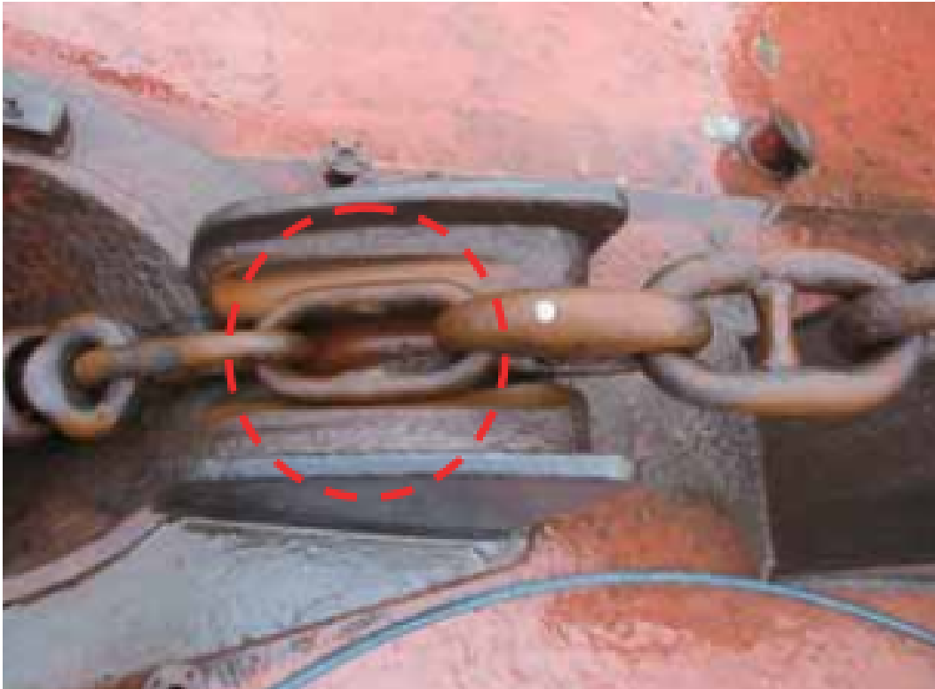
Worn link and missing of stud
