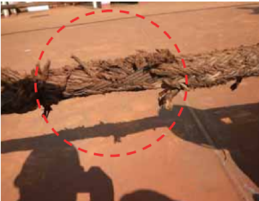
Deteriorated mooring line
