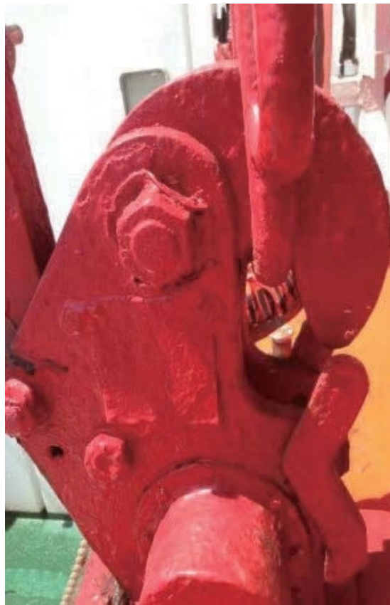
Seize of on-load release gear by excessive paint
