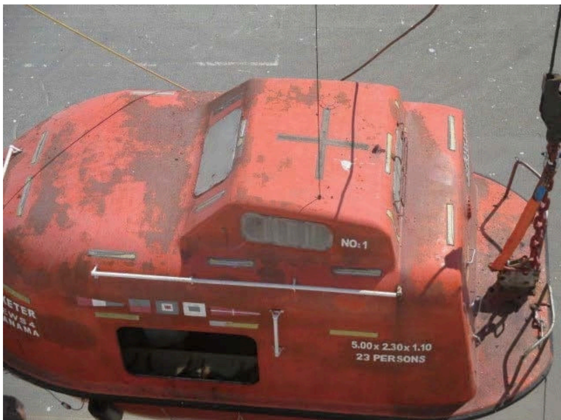
Seize of on-load release gear by excessive paint
