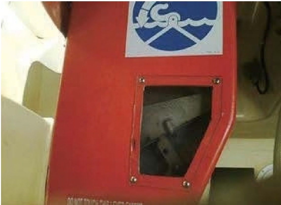
Improper reset of on load release gear interlock lever
