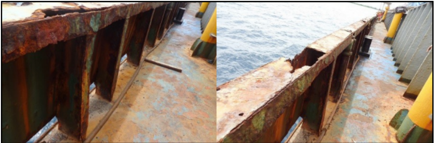
Damaged corrosion of Bulwarks and Freeing port
