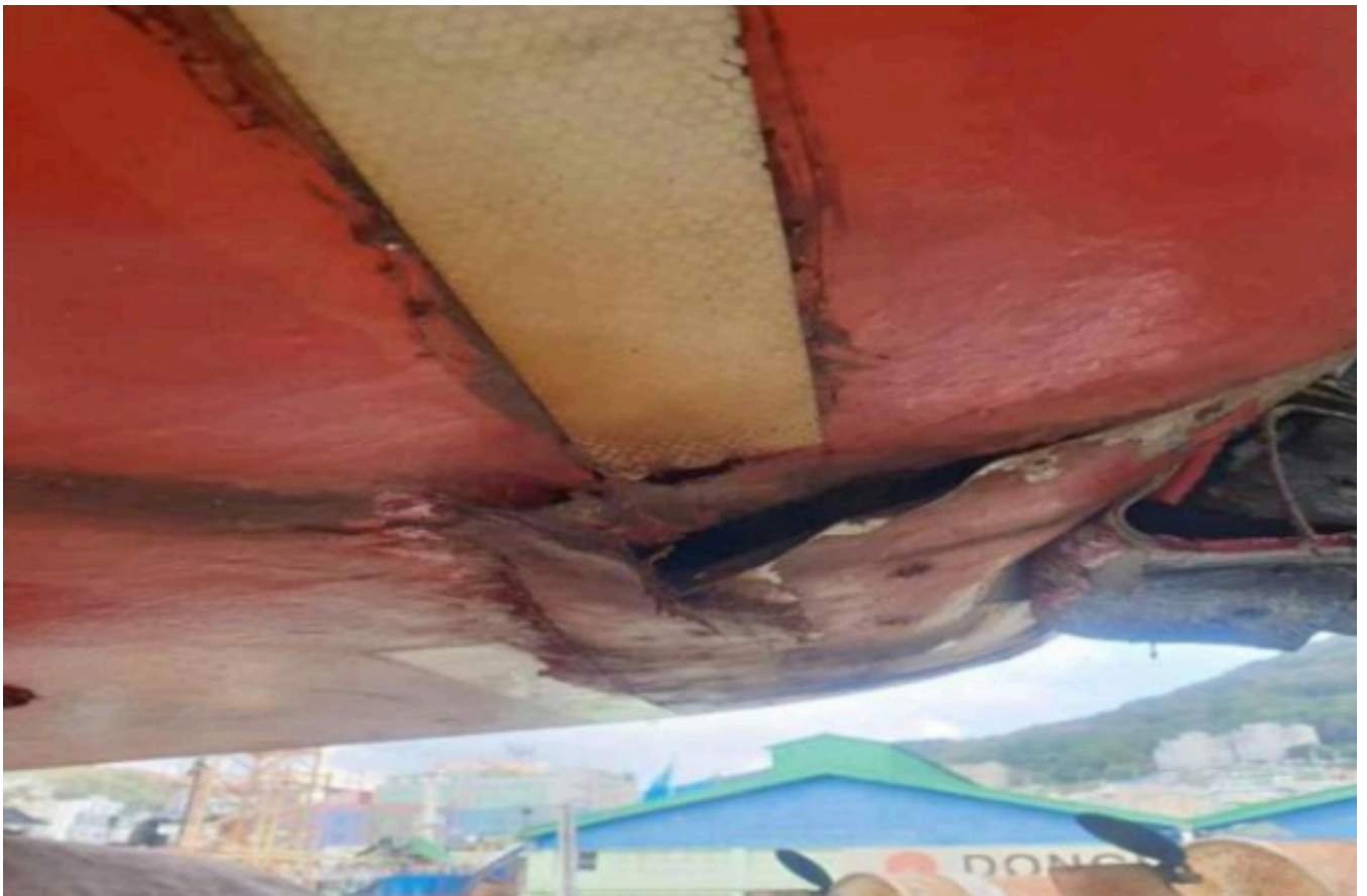
Rescue boat on boat-deck starboard side found hole on bottom.
