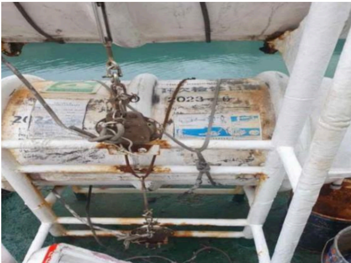
Inflatable liferafts not working properly - interval of serviced date exceed 12 months
