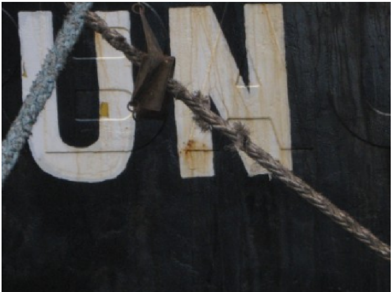
Bad condition of mooring rope.
